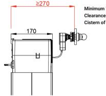
Minimum Wall Cavity Clearance for InWall Cistern of 270 mm
