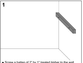
Screw a batten of 2" by 1" treated timber to the wall horizontally to support the bath rim. This ensures that the bath will remain stable and the rim cannot flex.
