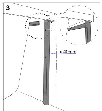
Screw another 2" by 1" treated timber batten vertically onto the wall, clamping the bath to the wall. This batten should be at least 40mm in from the corner of the bath. This batten will provide additional rim support. This should be done on both corners to securely hold the bath in place.
